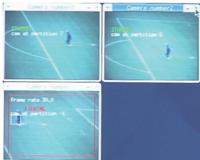
Figure 10 Tracking result 2 using 3 cameras; while the monitoring camera is filming the object, each of the stand-by cameras takes a position and waits for the target
