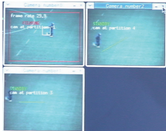
Figure 9 Tracking result 1 using 3 cameras; while the monitoring camera is filming the object, each of the stand-by cameras takes a position and waits for the target
