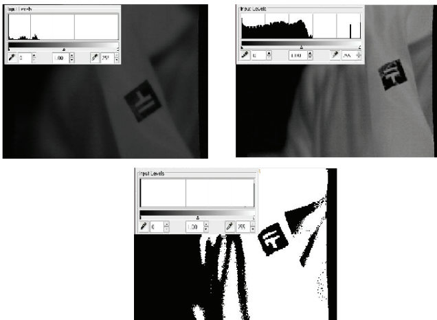
Fig. 6: Left: thermal capture without filter; Right: with contrast filter; Center: with threshold filter.
