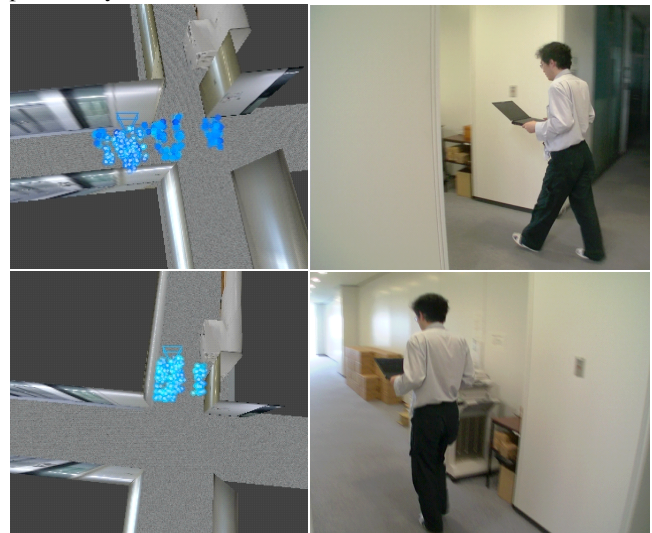
Figure 1. Map matching using a map converted from 3D environment model (Left-column presents probability distributions of locations of the user shown in right-column. Bottom-row presents the state one second before top-row).
