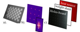
Figure 1: a). Chessboard image by LWIR camera using constant illumination. b). Image of holes-board by LWIR and the resoult of ellipce center location analysis of one hole. c).Holes-board with white sheet and heat source object constalation
