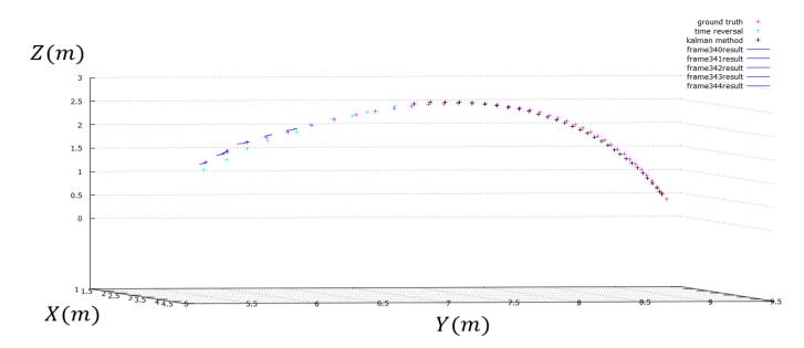
Fig. 5. Comparison experimental results of suggestion technique and the previous technique (3D position estimate of the shuttle)
