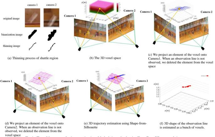
Fig. 4. Flow of the process of trajectory estimation of the badminton shuttle using Shape-From-Silhouette technique
