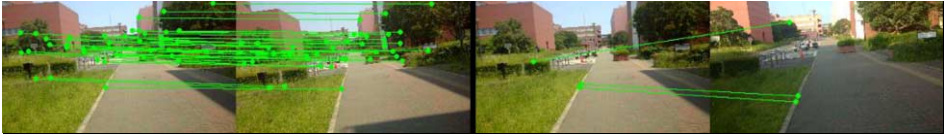
Figure 1. SIFT key pair (left: small gap in time and space, right: large gap in time).
