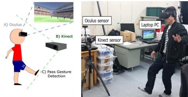
Figure 2. System Setup. Left: reference system configuration: A) The user experiences the VE through Oculus CV1. B) Kinect tracks the user’s body. C) When a passing gesture is detected, the passing action occurs inside the VE as well. Right: A user experiencing the VR soccer simulation.
