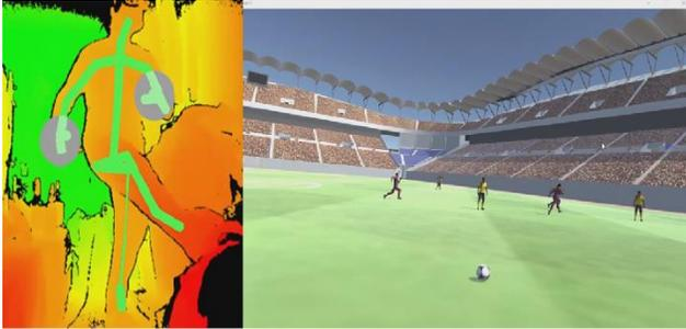
**Figure 3. Passing Gesture Action. Left: the image detected by the Kinect of a user performing the passing gesture. Right: the ball pass is triggered as a result inside the VE.**
