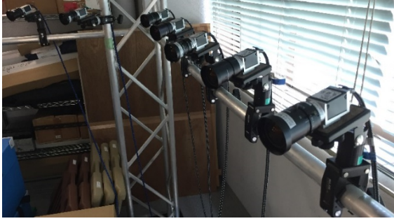
Figure 6: An overview of camera setting. 20 multi-view cameras are placed in a U-shape
