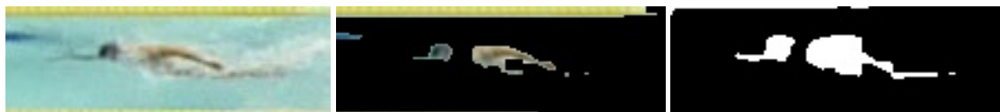
Figure 8. Swimmer region. From left to right, a segment that includes main part of the foreground region, its binary representation, and its color representation.
