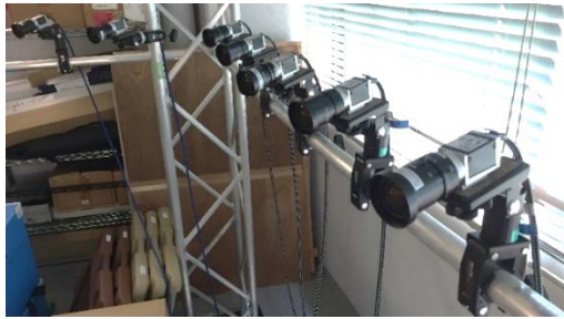
Figure 12: An overview of camera setting. 20 multiple viewpoint cameras are placed in a U-shape.
