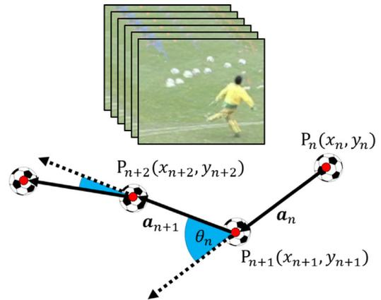
Fig. 8. In all of the input and interpolation images, we acquired the observation position of the object. Next, we calculated the angle  $\theta_n$  between the following two vectors.
