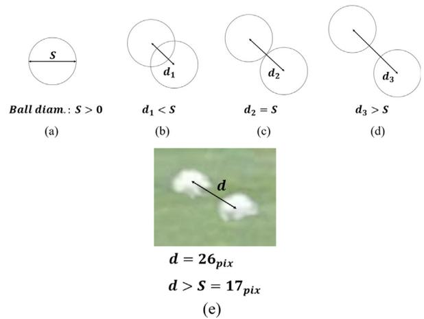
**Fig. 13.** (a) Soccer ball diameter:  $S$ , (b-d) The distance between the ball centres in the two frames:  $d$ , and (e) The distance  $d$  of the experimental environment.
