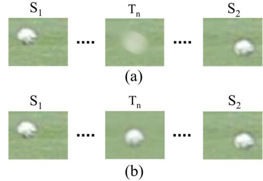
Fig. 7. (a) Initial interpolation image after applying the motion blur effect. (b) Interpolation image generated using the initial interpolation images.
