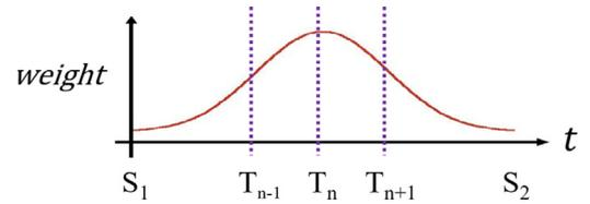
Fig. 6. The blend ratio of the subject and the background is determined based on the interpolation distance between the two input images using the normal distribution.
