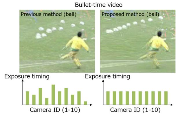
**Fig. 2.** Result derived from the comparative task that applies combined processing methods to all camera sequence images. Left: When a bullet-time image is captured using multiple asynchronous cameras, the observed position of the ball moving at a high speed deviates because of the effect of the synchronisation deviation. Right: In the proposed method, the deviation is reduced through frame interpolation processing and a smooth viewpoint switching image is generated.
